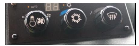
The system shall control the temperature of the cab and crew cab automatically by pushing the center of the fan speed control knob. Rotate the center temperature control knob to set the cab and crew cab temperature.
